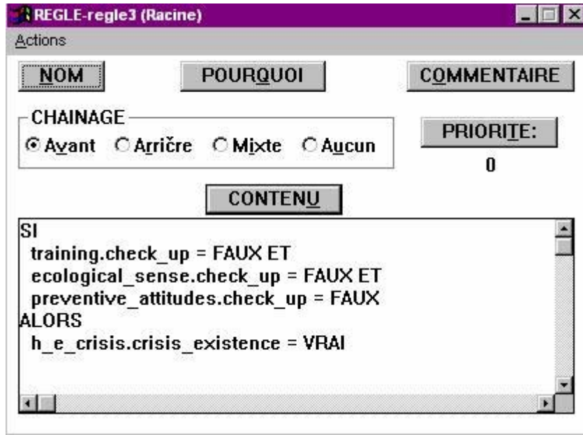
Figure 5. The rule that triggers the activation of the Human Operator-Environment Crisis Class
