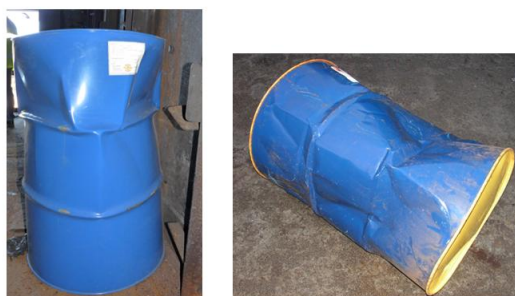
Figure 6: An oil drum (left) after it has exposed to a deflagration loading of 1.4 bar and duration of 110 ms (centre) and one exposed to an overpressure of 1.8 bar with a duration of 43 ms (right).
