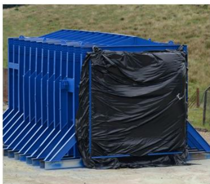
Figure 3: A picture of the bang box and an example of pressure-time profile produced in one of the tests. The vent area of the bang box is shown covered for protection of the internal equipment against the environment.
