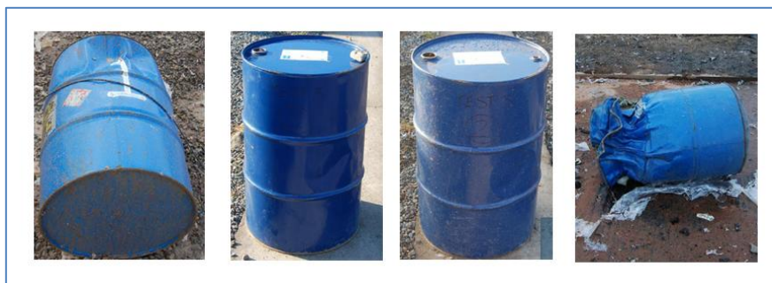
Figure 5: Drums exposed to shock loading of a range of pressures and durations. The one on the far right was inside a detonation cloud. For the three on the left and from left to right, the maximum incident overpressures were 4.4 bar, 2 bar, and 0.4 bar and the respective durations were 10 ms, 11 ms and 15 ms.
