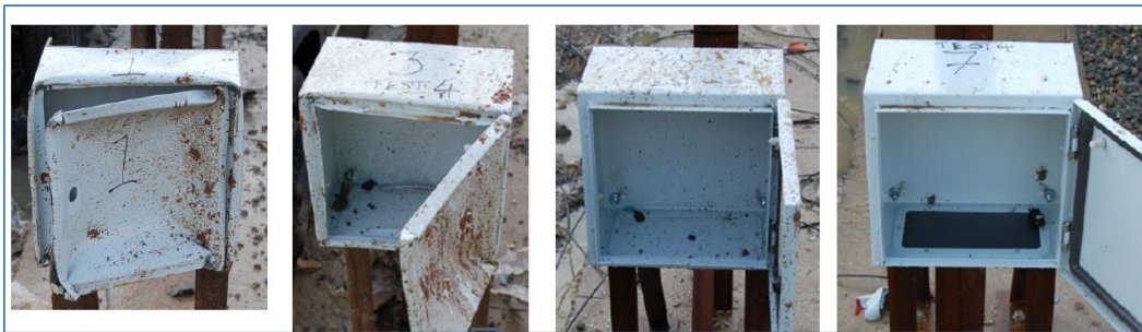
Figure 4: Switch boxes exposed to shock loading of a range of pressure and durations. The incident overpressures were (from left to right) 8.2 bar, 3.4 bar, 2.1 bar and 0.7 bar. Duration ranges from 4 ms to 10 ms.
