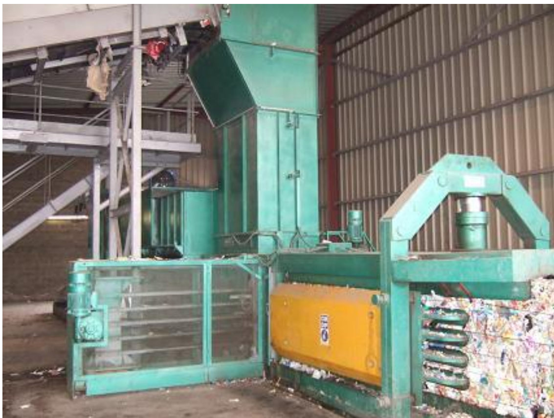
Figure 1. View of a crushing press used for aluminum waste recycling.
