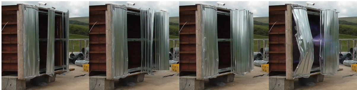
Figure 10: Video stills of the venting event showing panel failure in Test 10
