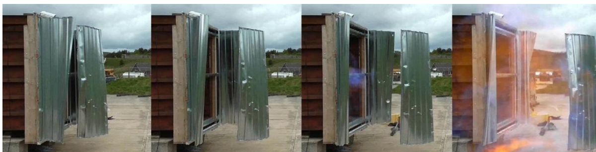
Figure 9: Video stills of the venting event showing panel failure in Test 8
