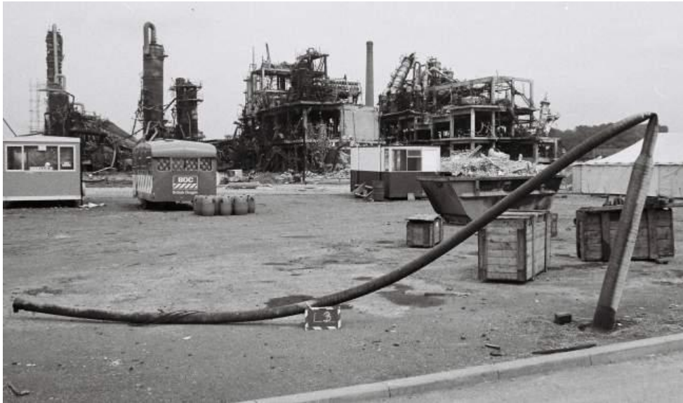
Figure 19: Lamp post within the cloud – approx. 130 m (426 ft) south of vapour source.
