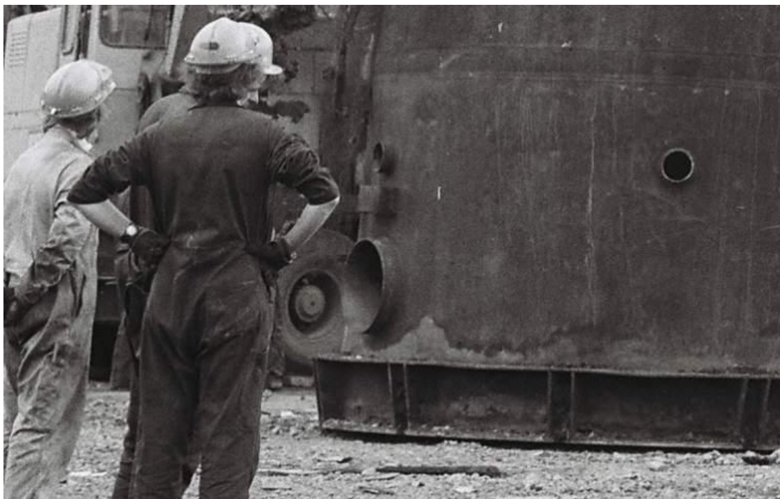
Figure 10- Reactor 2: Limited pressure damage to reactor skirt
