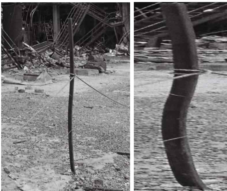
Figure 16: Curved fence posts in open areas to the south of the cyclohexane oxidation plant.
