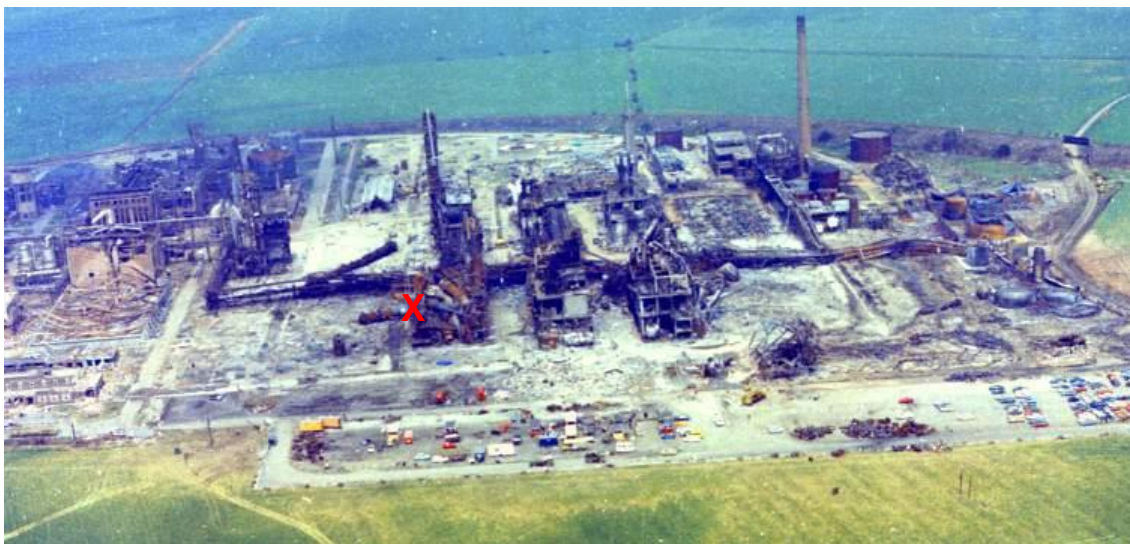
Figure 5: Aerial view of the Flixborough site after the incident – release point marked X
