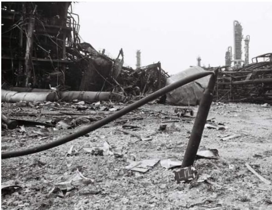
Figure 20: Lamp post within the cloud – approx. 180 m (590 ft) NE of vapour source
