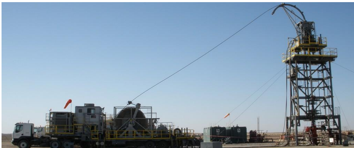
Figure 1: Coil Tubing Rig Up
