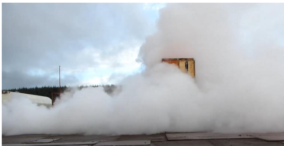
Figure 4: Side view of the interaction of the dispersing plume with the containers
