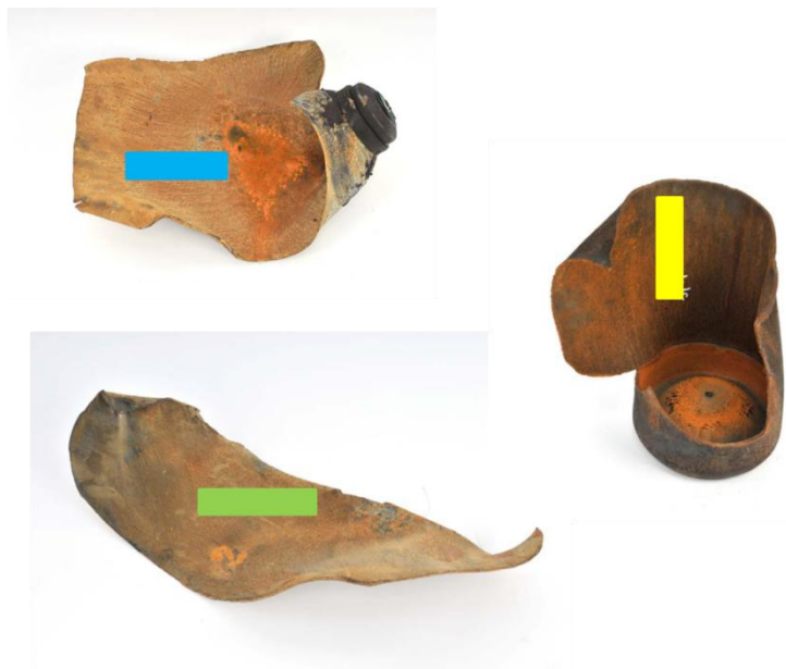
Figure 2. The three fragments of the incident cylinder - colours relate to flight paths shown in Figure 3
