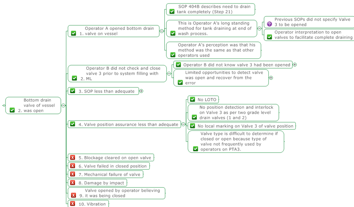
Figure 2: Example section of logic tree related to the valve being left open. HFAT® output was used to inform the behaviours of Operator A opening the bottom vessel valve and Operator B not closing the bottom vessel valve.
