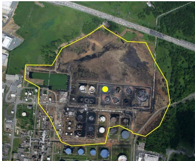
Figure 1: Burn pattern left by a gravity-driven vapour current – source marked by circle
