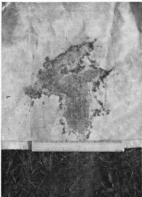
Fig. 9.—Close up of damaged fabric
