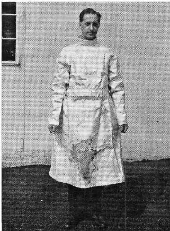
Fig. 7.—Coat damaged by splash of burning sodium
