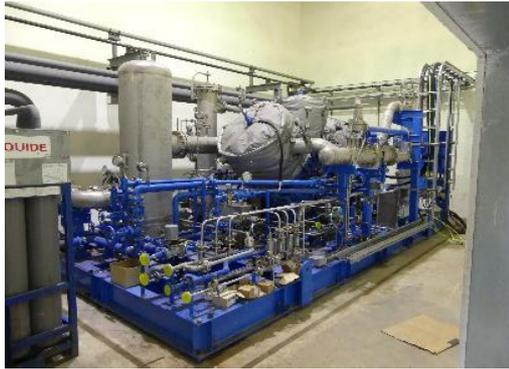
Syngas compressed to high pressure. Demonstration plant use 3 stage reciprocating compressor to take gas to 15 bar.
