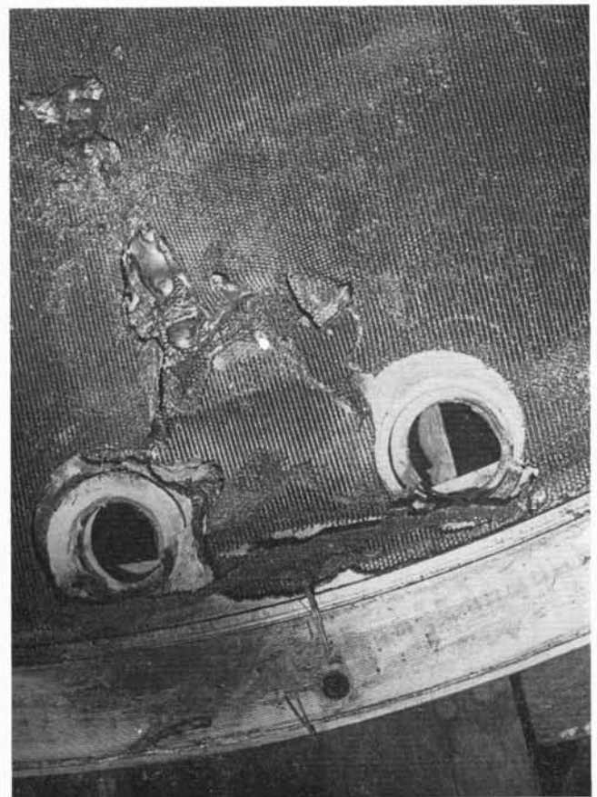
Fig 5 Cell 16/3 showing damage to electrodes and asbestos separator
