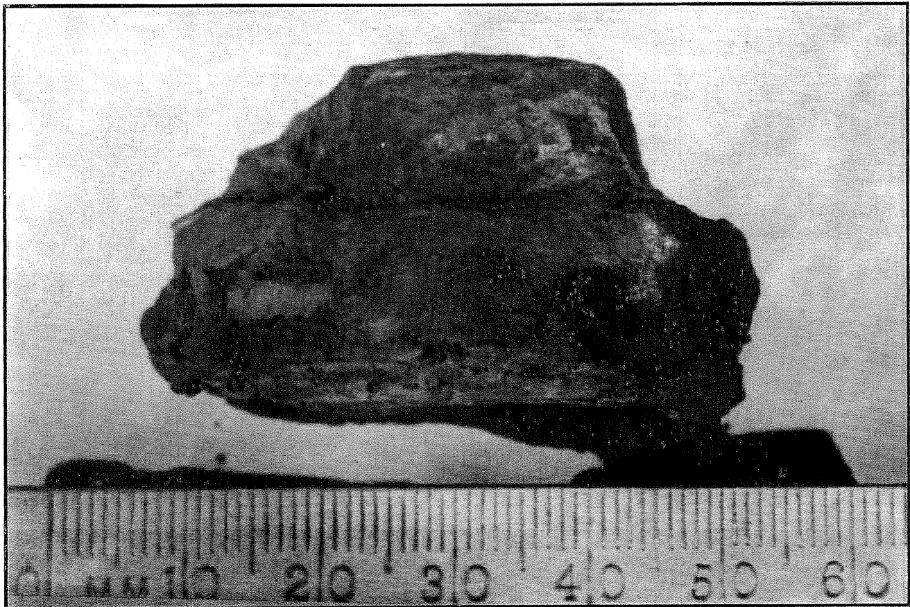
Fig 1 Corroded plug before surface non-metallic material was removed
