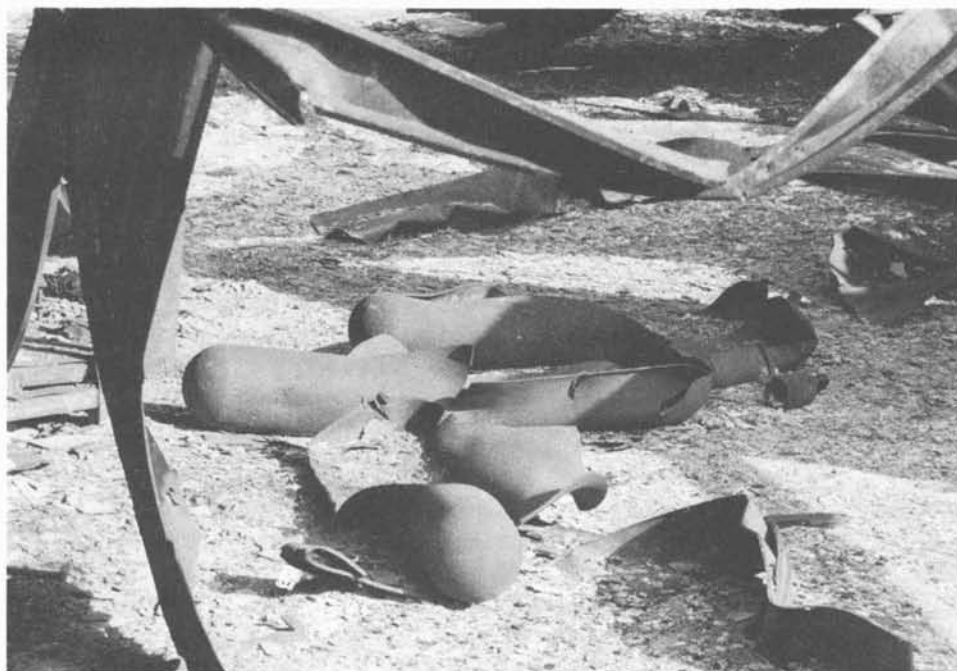
Exploded acetylene cylinders in Unit 5
