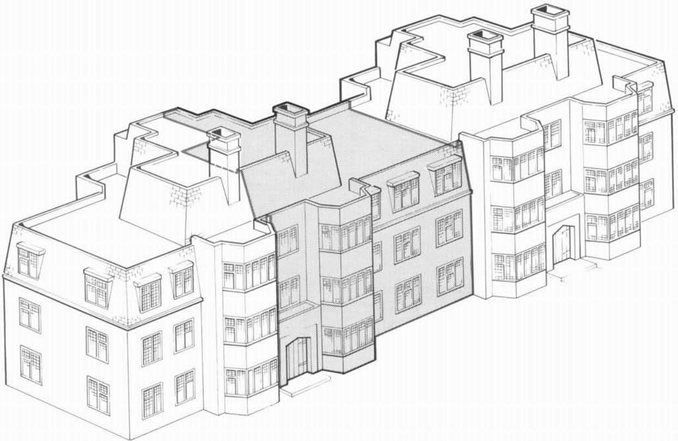
Fig 2 Area of Newnham House destroyed by explosion
