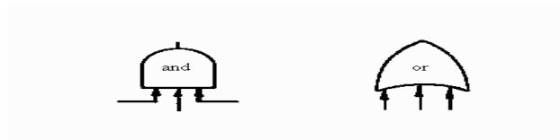
Figure E 6.2.1 The symbols for “and” “or” logic
