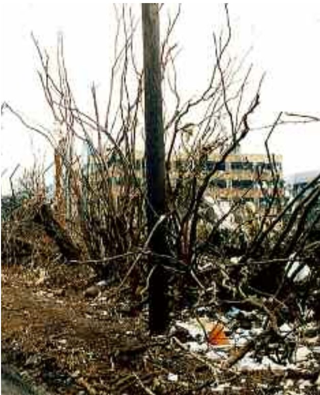
Figure 7 A telegraph pole in Buncefield Lane, showing sooting on lower half
