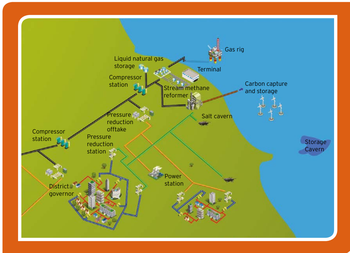
Figure 6: The h21 Leeds City Gate project will aim to decarbonise the district heating network of Leeds, UK, linking hydrogen fuel production to a local CCS network Source 84 .
