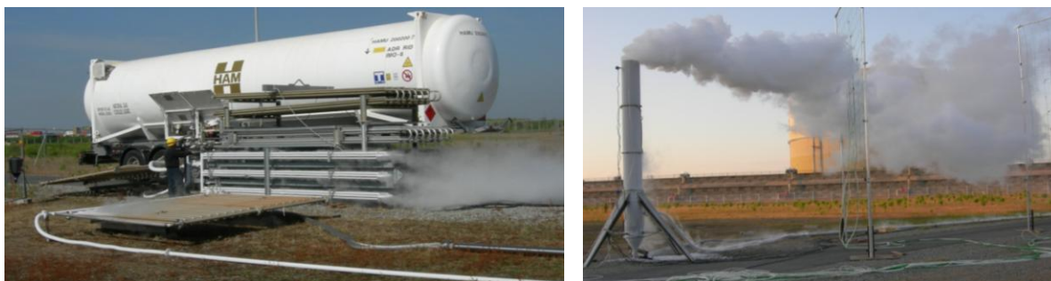
Figure 1. LNG vapour generator (left) and LNG vapour release through the vent (right) used during the experimental campaign.
