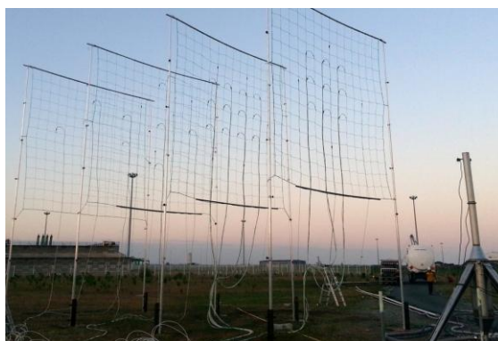
Figure 2. movable screens fitted with temperature sensors, and aspirating probes linked to oxygen meters and methane analysers.
