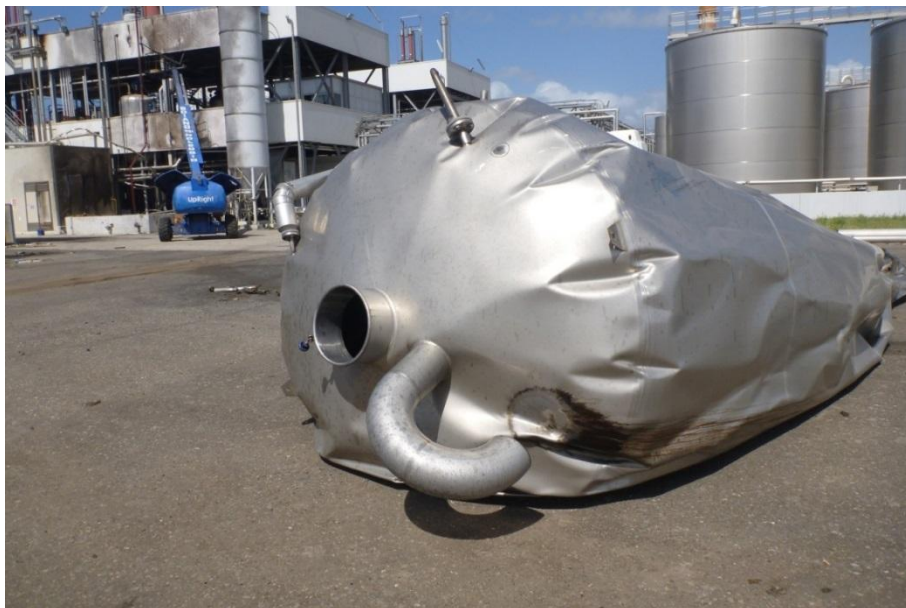
Figure 10: the tank landed 60 m away from its original location in the backstage close to the blue lifting machine.
