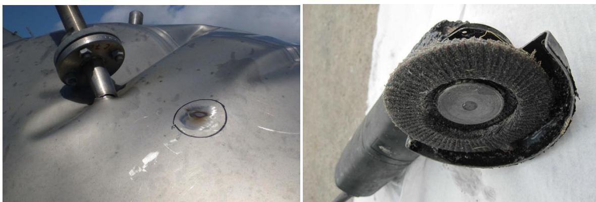
Figure 11: scrap on the tank roof and the tool used at the moment of the accident
