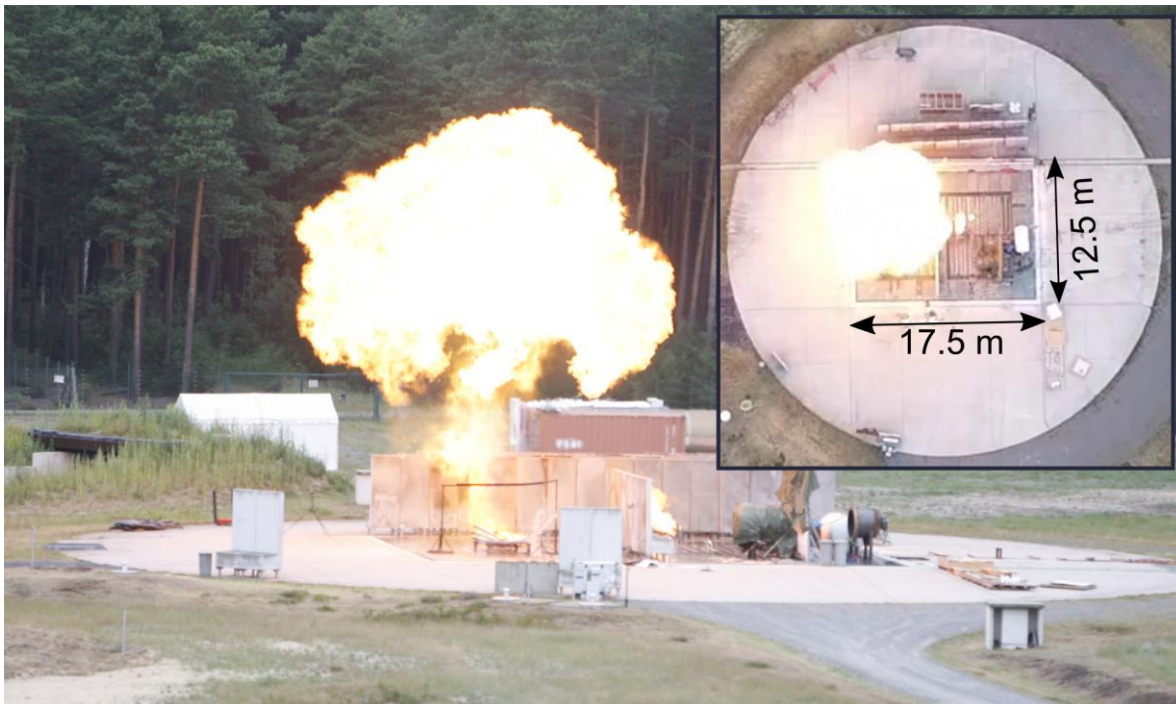
Fig. 3: Exemplary view on the fireball after failure of the gas vessel on the propane burner test bench (test pc12), side view and aerial view
