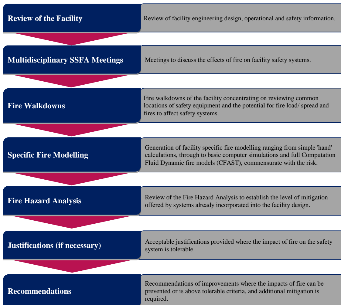
Figure 5 - Safety System Fire Analysis Process Flowchart
