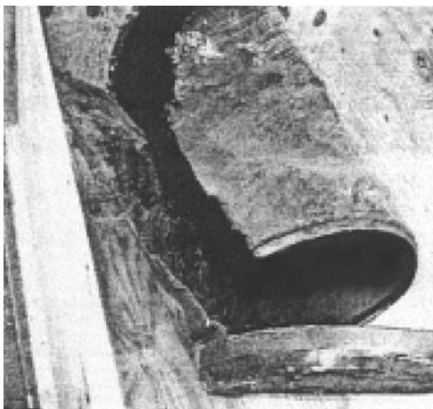
Figure 4. Ruptured 55-gallon plastic drum found in the area of origin.
