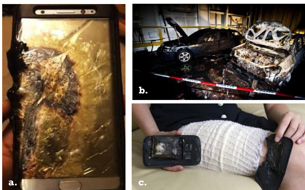
Figure 1 lithium-ion batteries fire and explosion incidents. (a) Samsung Galaxy Note 7 (2016)). (b) Electric Cars after fire in 2010 (Marlair and Lisbona 2012). (c) Samsung Galaxy S3 (Grabert 2013).
