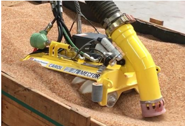
Figure 11: Sorbead WS 2050, 625 kg/m 3 (39 lb/ft 3 )
