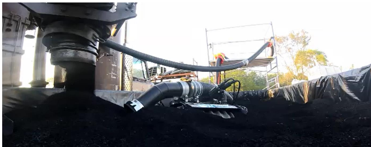
Figure 15: Endurance test with material recirculated back into the reservoir
