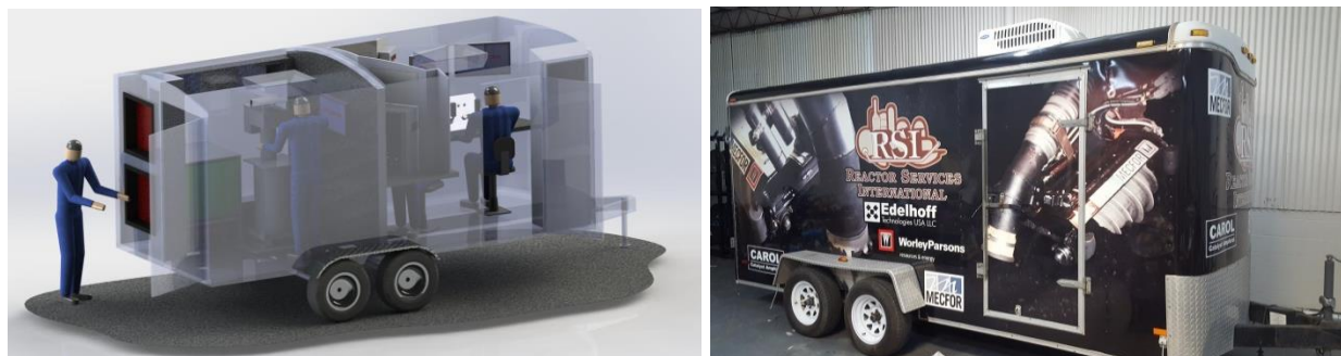
Figure 5: Control systems located in an air conditioned trailer
