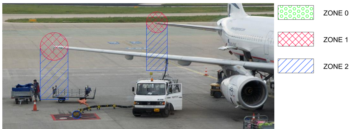
Figure 3 – Aircraft Wing Vent Zoning
