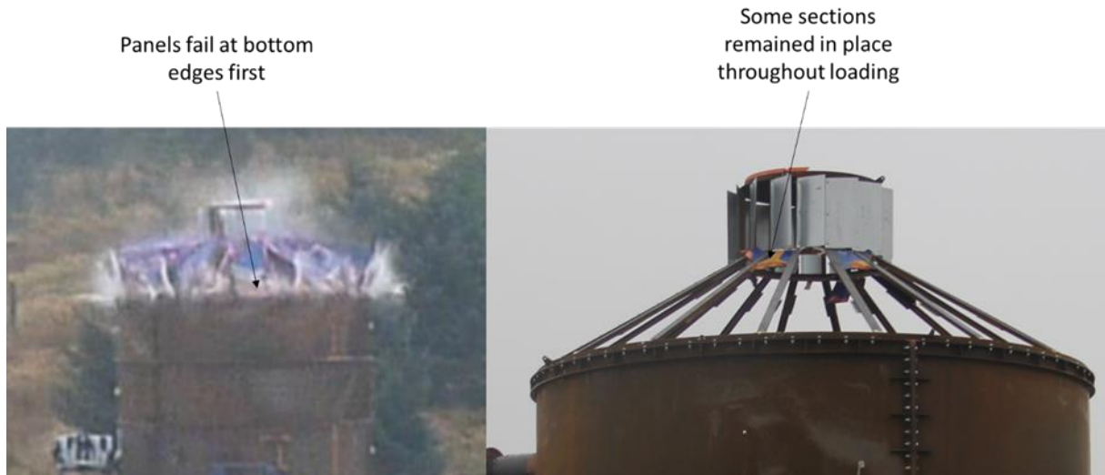
Figure 12: Test 7A – Frangible Roof Following Test
