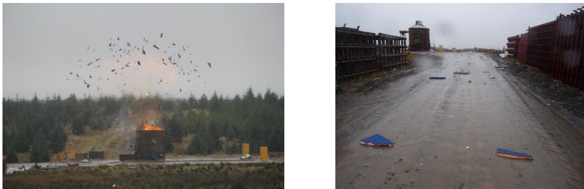
Figure 11: Test 7 – Frangible Roof Test
