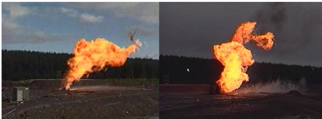
Figure 5 Examples of puncture fires in clay (left) and sand (right)
