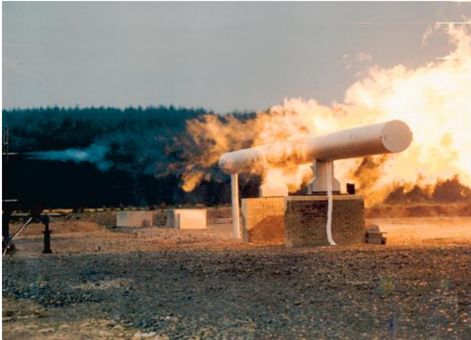
Figure 6 Example experiment measuring heat loading with a jet fire
