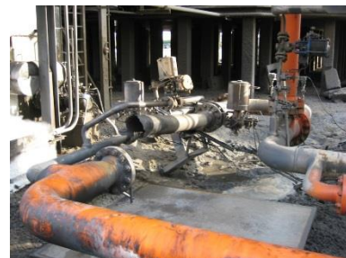
Figure 11: Internal deflagration in a pipe, failure near ultimate pressure - 25 projectiles found 0.1-1.7kg, 10m to 140m. Secondary projectile of structural support moved 8m
