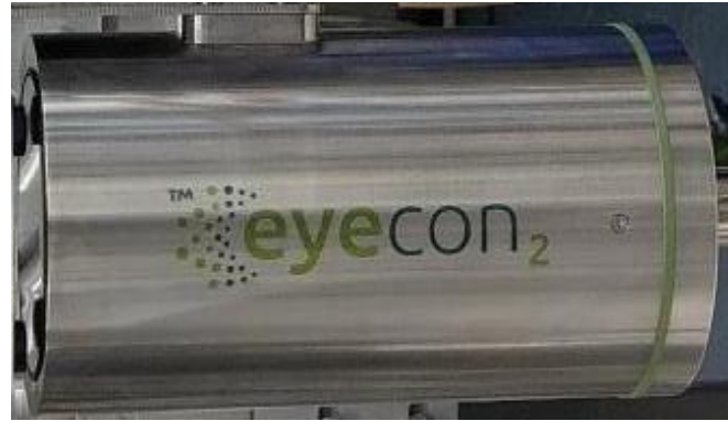
Innopharma Eyecon2 Particle Analyser
