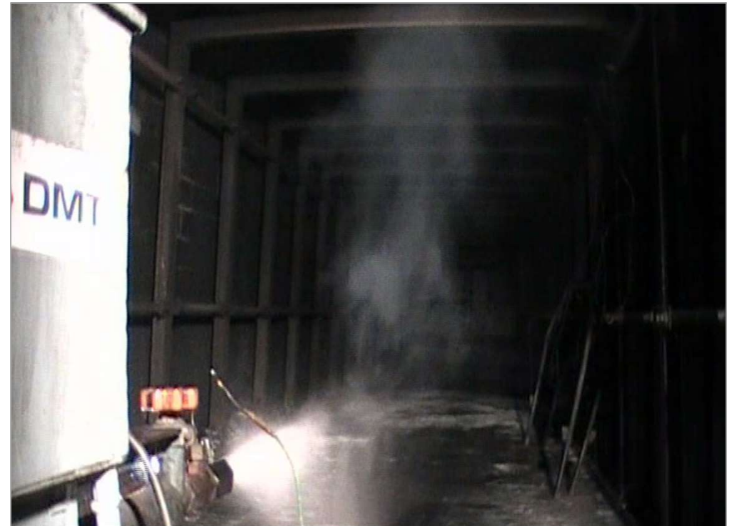
Synthetic Ester. Nozzle temp 120 °C
