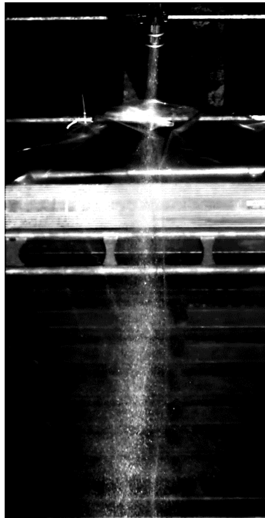
Figure 49 left: Test 1 – 1.0 m axially from release (pressure 4.19 bar g)
