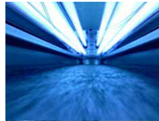
Inside view of the supercritical UV device. Two UV bulbs are in the lid seen at the top of the photo, with the supercritical flow in the open channel at the bottom of the photo (left), racked 8-module supercritical UV system (below).
