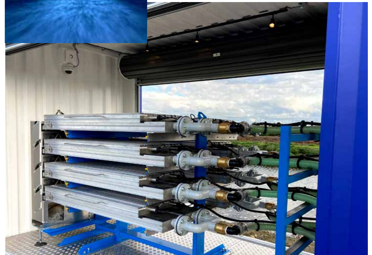
Inside view of the supercritical UV device. Two UV bulbs are in the lid seen at the top of the photo, with the supercritical flow in the open channel at the bottom of the photo (left), racked 8-module supercritical UV system (below).
