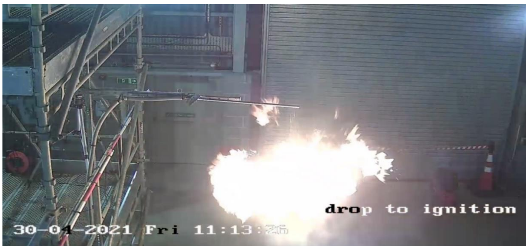
Figure 15: CCTV image 5 - Test 79 Axial 4.75 m ignition position
