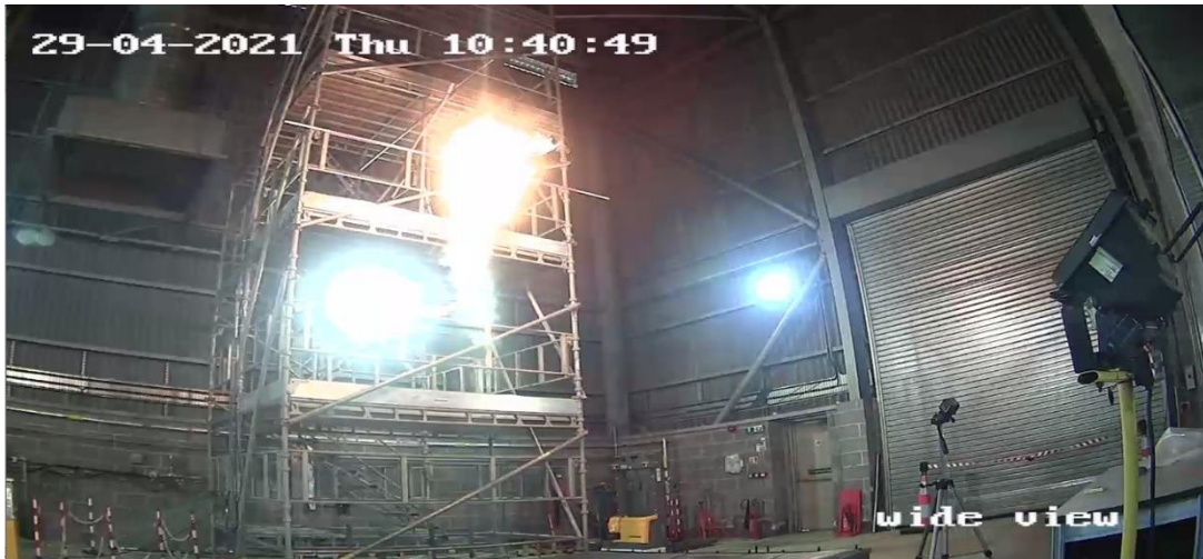
Figure 11: CCTV image 5 - Test 64 Axial 2.9 m ignition position
