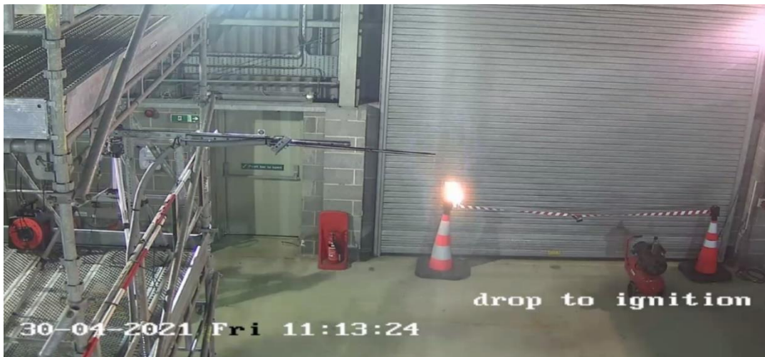
Figure 14: CCTV image 1 - Test 79 Axial 4.75 m ignition position
