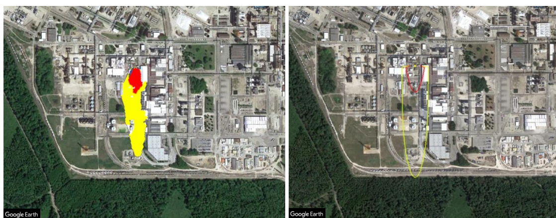
Figure 7: Case 3 dispersion modelling results, CFD (left) and Gaussian (right), ground level effects.
