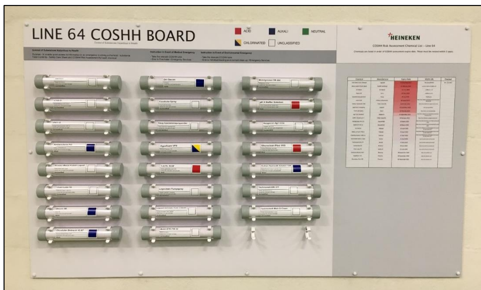
Figure 2: An example of a COSHH Board with COSHH tubes on one of the Heineken UK production lines
