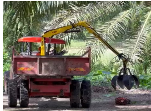
Figure 2: Picture shows integration of machineries, palm oil grabber in picking up the Fresh Fruit Bunch.
