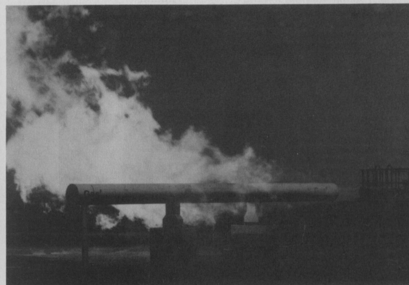
FIG. 1 - A 10 kg/s natural gas flame impinging on an instrumented pipe target
