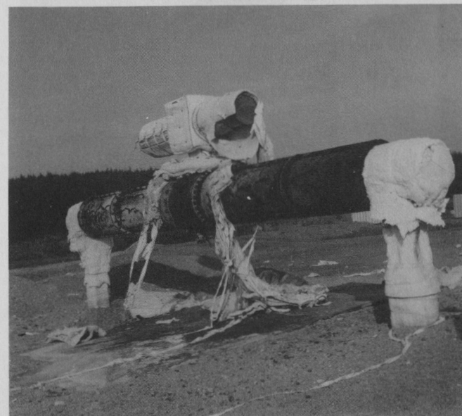
FIG. 5 - One of the soft-jacket protection systems, before and after testing
