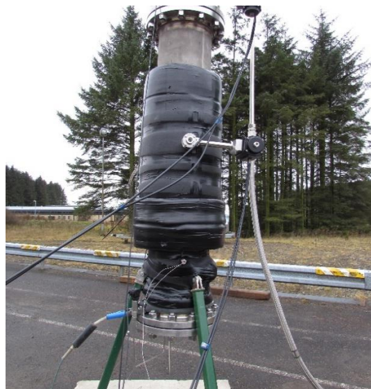
Figure 1: Experimental rig for Test 2. The outer stainless steel surface is lagged to improve the thermal insulation
