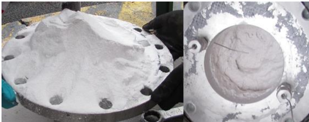
Figure 6: Perlite collected (left) and the bottom surface of perlite (right) after completing Test 4. The perlite void extended approximately 100 mm into the chamber
