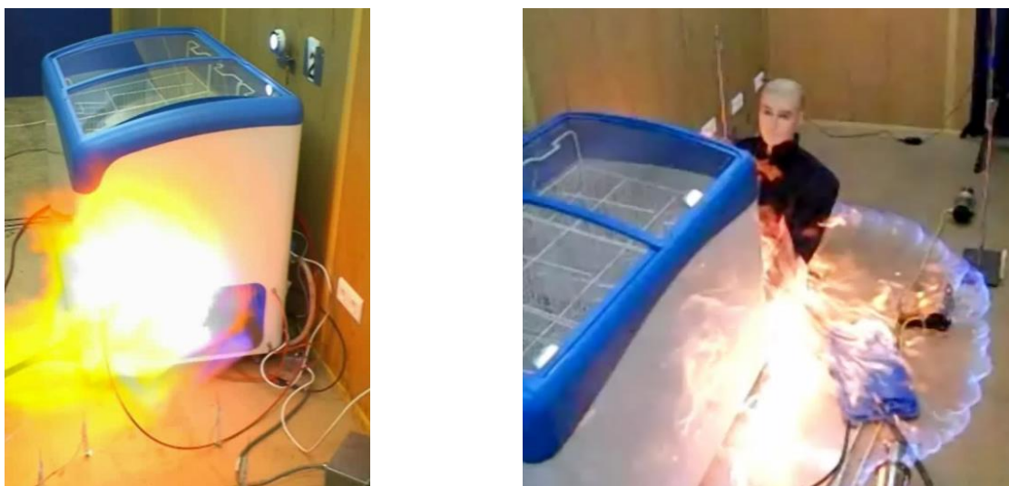
Figure 8: Ignition tests involving commercial refrigerated cabinet
