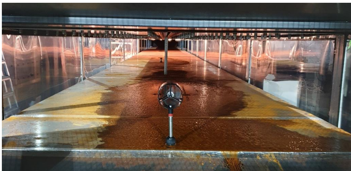
Figure 6 View down the tunnel with anemometer, sampling boom and propane inlet slightly offset from the center axis.
