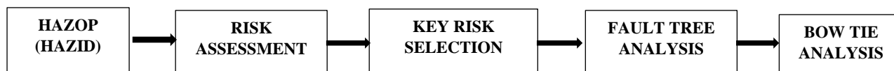
Figure2 Analytic Studies used in the Hazard and Risk Analysis on the Copper Processing Plant
