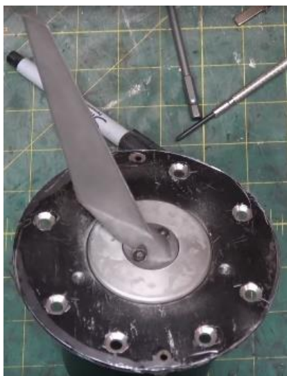
Figure 7: Typical angle-of-attack sensor
