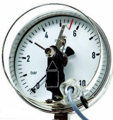
Figure 11: Analogue pressure gauge and alarm
