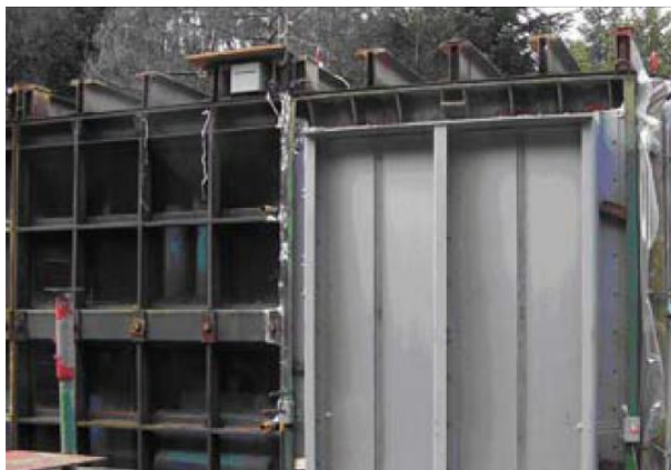
Figure 9 Explosion Relief panel before explosion test
