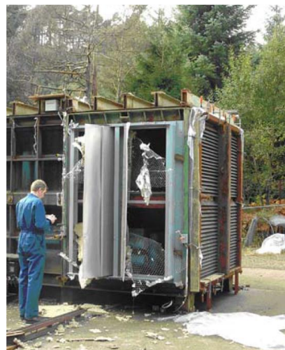
Figure 10 Explosion Relief panel after explosion test to 0.5bar.
