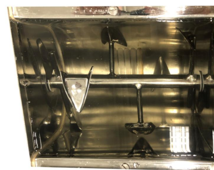
Fig 1. Geometry optimisation of a ploughshare mixer used in industry to mix pastes and powders. CFD simulations validated using Positron Emission Particle Tracking/Projection Imaging. CAD optimised for mixing efficiency using HARPPP.
