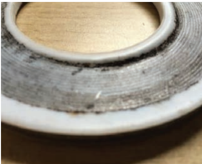
Overtorqued PTFE envelope gasket
