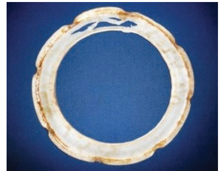
Over compressed PTFE gasket due to over torquing of bolts
