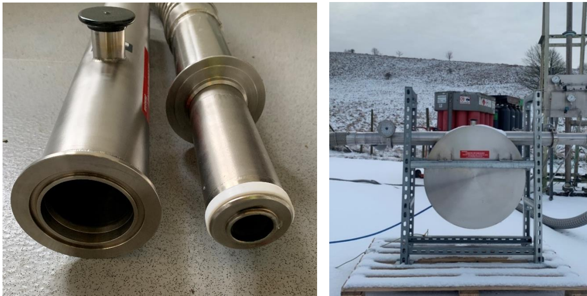
Figure 6: The left picture shows a 1.5" Linde bayonet and the corresponding female port (note that these are not the bayonet and port pair that leaked, but are shown for illustration). The right picture shows two joints held in place by the clamp
