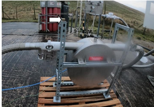
Figure 5: Ice can be seen on the joints of the hoses with the flowmeter after the experiment has finished. The vacuum plug is no longer in the port and is marked with the arrow on top of the frame
