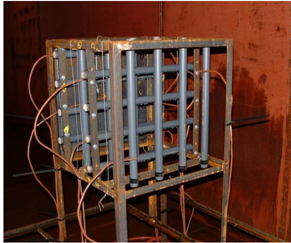
Figure 1: HSE JIP Testing Congestion
