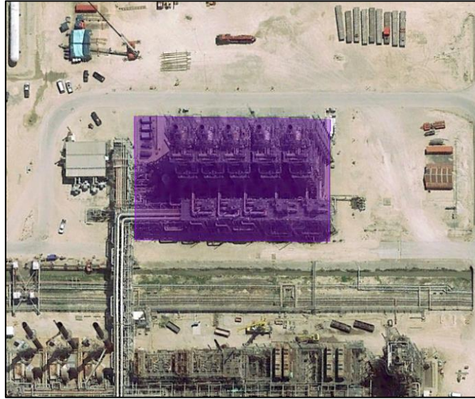
Figure 5. Case Study 2- Fire area defined for a fired heater unit based on CCPS guidance
